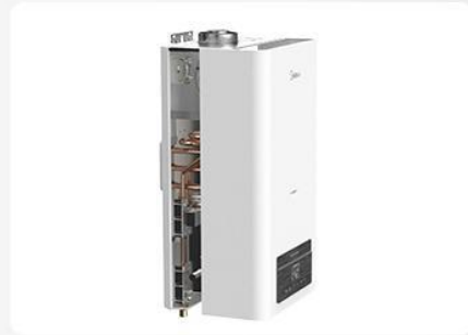
Unscrew 4 Screws to Remove the Shell
